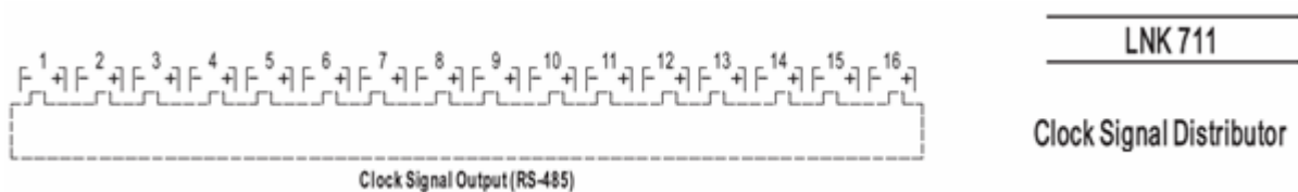
Figure 3-4 Connection diagram of signal output terminal of LNK711
